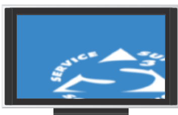
Figure 2: The source resolution does not match that of the display, resulting in a fuzzy, distorted image.
