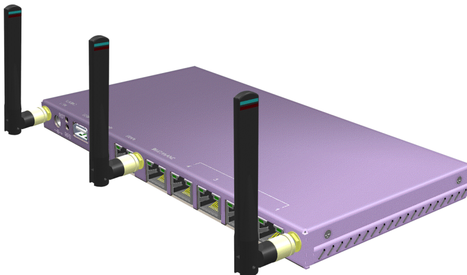
Optional IEEE 802.11n Wireless LAN with 3 antennas
